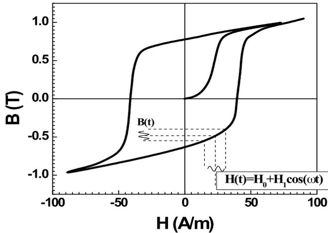
Fig.1 Typical hysteresis loop of the magnetic material
