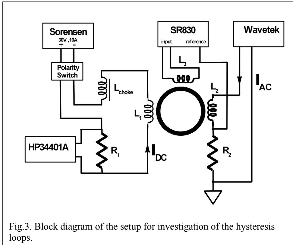
For measurement of the magnetic permeability we will use the setup shown in Figure 3. The bias magnetic field in the toroid is generated by driving a DC current through the primary coil  $L_1$ . The current is supplied by the Sorensen power supply, which can provide a maximum
